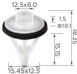
C1615 Material: POM Color: White Tailgate panel
