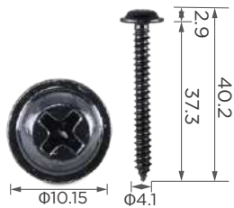
H2229 Head style: Phillips truss Position: Genuine screw Metric: M8
