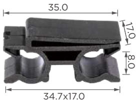
C1212 Material: POM Color: Black Tube & cable routing clip
