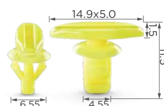
C1505 Material: POM Color: Yellow/ Natural Bonnet weatherstrip, front and rear door weatherstrip
