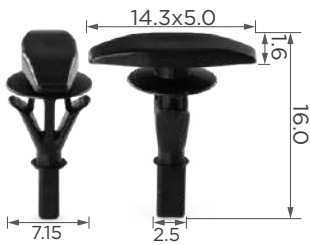
C0035 Material: POM Color: Black Front and rear door weatherstrip
