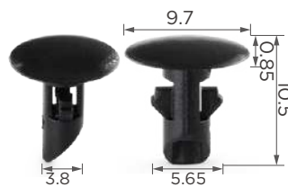
C0590 Material: PA Color: Black Front and rear door weatherstrip
