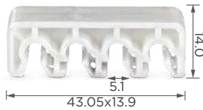
C1376 Material: POM Color: White Tube & cable clip
