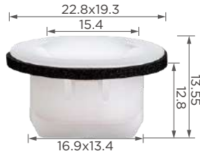
C3774 Material: POM Color: Natural Front and rear bumper
