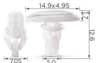
C1501 Material: POM Color: Natural Front and rear door weatherstrip
