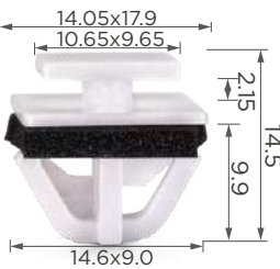
C1697 Material: POM Color: White Side moulding, rocker panel
