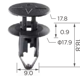
C1887 Material: PA Color: Black Front and rear bumper, engine cover, grille
