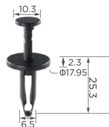
C0047 Material: PA Color: Black Dashboard, rocker panel, front and rear fascia, quarter panel
