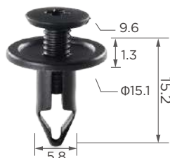
C3383 Material: PA Color: Black Expanding retainer
