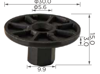
C3720 Material: PA Color: Black Wheelarch, fender liner
