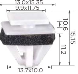
C1637 Material: POM Color: White Front bumper
