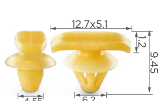
C1788 Material: PA Color: Yellow Front and rear door weatherstrip
