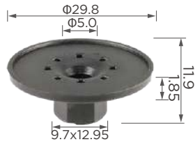
C3433 Material: POM Color: Black Fuel tube, front floor
