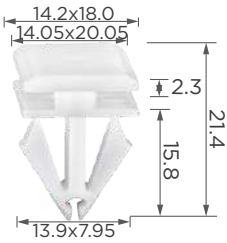
C1604 Material: POM Color: White Side moulding, rocker panel
