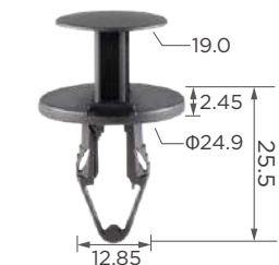
C3368 Material: PA Color: Black Mud shield
