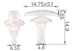
C0247 Material: POM Color: White Front and rear door weatherstrip
