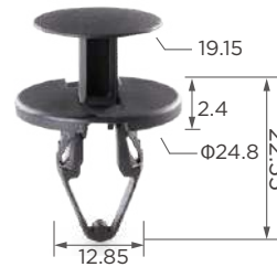
C3363 Material: PA Color: Black Front and rear bumper, dashboard, air conditioning
