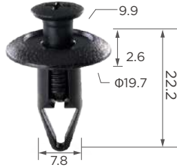
C1914 Material: PA Color: Black Front bumper, front end, wheelarch
