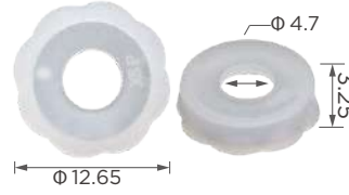
C3857 Material: PA Color: Natural Pop-on screw cover base
