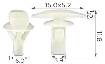
C0607 Material: PA Color: White Front and rear door weatherstrip, hood
