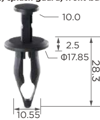
C1948 Material: PA Color: Black Expanding retainer
