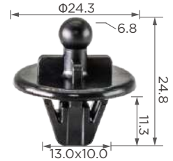
C3716 Material: POM Color: Black Rear tray, Parcel shelf fixing strap pin
