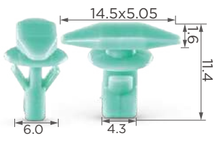
C0628 Material: POM Color: Green Instrument & side panel clip
