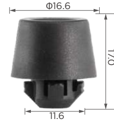
C3766 Material: TE Color: Black Hood / bumper stopper
