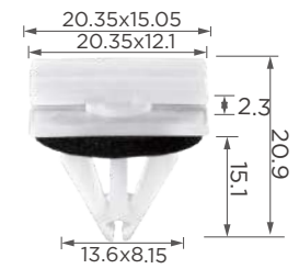
C1626 Material: POM Color: White Side moulding, rocker panel
