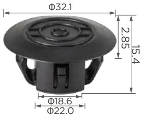
C3689 Material: PP Color: Black Rocker panel, side molding
