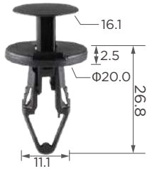
C3342 Material: PA Color: Black Underbody panel & firewall insulation
