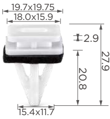
C1524 Material: POM Color: White Side moulding, rocker panel
